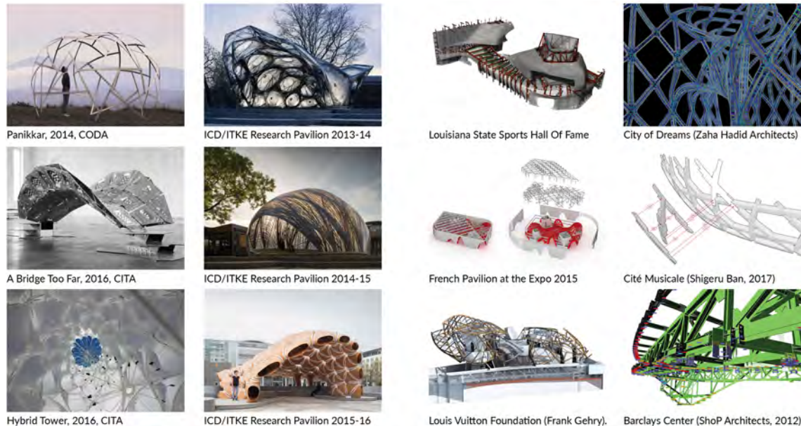
Figure 3.13: This figure highlights the difference between the material specific and seamless design integration of research pavilions and demonstrators in academia (left), and the heterogeneous design landscape of the building industry (right): element clashes, intricate material interfaces, large diversity of employed materials, etc.
