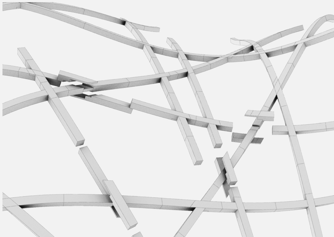
Figure 4.10: Generation of networked lap joints.
