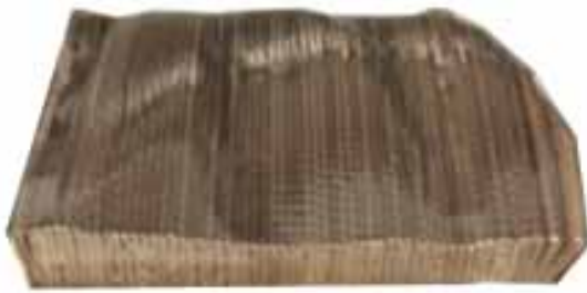
Figure 2: Plexi Vacuum formed on cardboard (Smith 2014)
