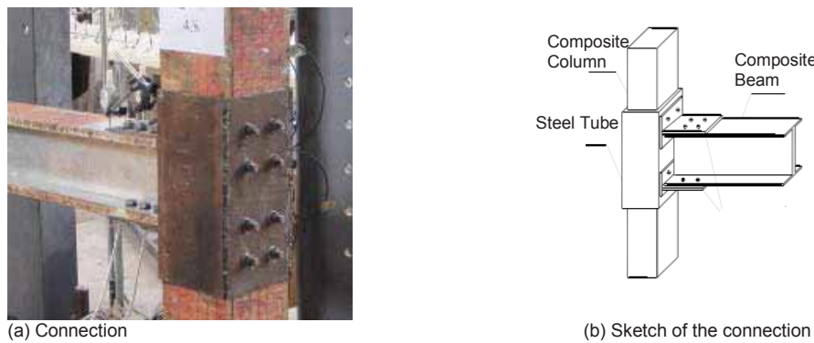
Figure 6: Connection for bamboo-steel composite beam and column.
