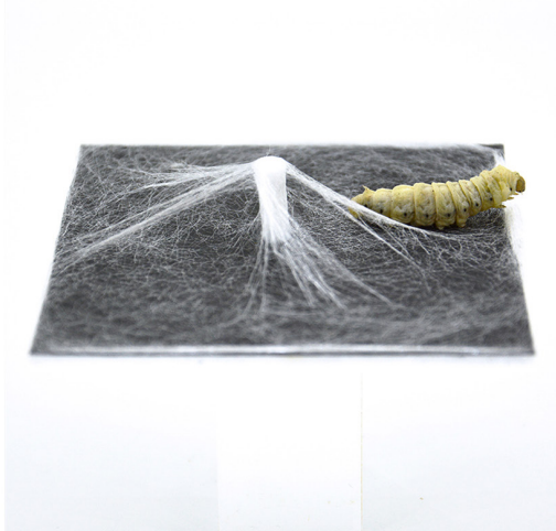
Figure 6 18mm one-dice platforms illustrating higher density deposition along the shortest distances from the geometrical center to the surface boundary contour.
