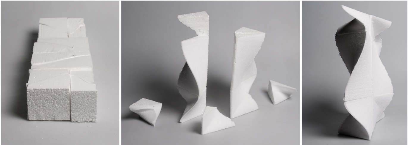
8 Highly-material efficient fabrication of spatial structures through flank milling in 2010.
