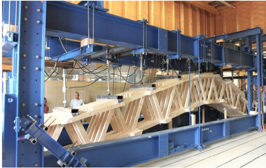
Fig. 10. Full-size load tests of automatically prefabricated lattice girders with a regular span of almost 15 m at the Bern University of Applied Sciences (Image ©Arch-Tec-Lab).
