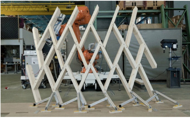
Fig. 4. Initial robotically built prototype based on a material-efficient construction typology developed by Friedrich Zollinger during the beginning of the 20th century. Gramazio Kohler Research, ETH Zurich, 2012.
