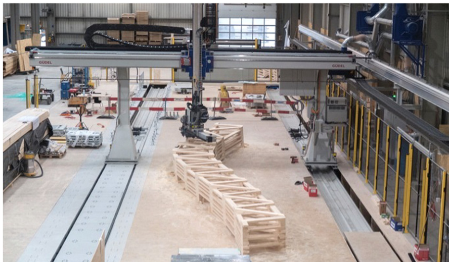
Fig. 9. Custom six-axis overhead gantry robot of ERNE Holzbau AG, featuring a translational axis with a mechanical wrist and three additional rotational axes to perform fully automated fabrication tasks within an effective workspace of 48 \times 6.1 \times 1.9 m (Image ©Arch-Tec-Lab).
