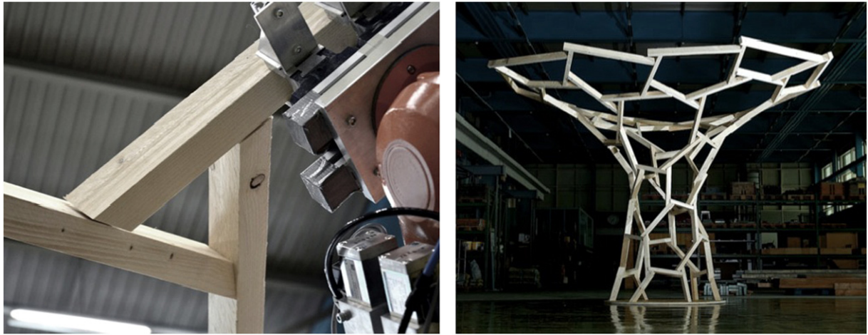
Fig. 6. Left: custom-developed spatial node connection for spatial robotic assemblies – by increasing or decreasing the size of its triangular arrangement, the stiffness of the connection can be individually adapted to specific local structural requirements; right: final 1:1 prototype, testing the feasibility of the connection according to tolerance compensation, structural performance and design freedom. Gramazio Kohler Research, ETH Zurich, 2014.
