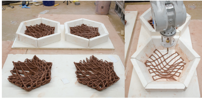
13 Porous ceramic tiles composed of bridged and looping clay beads.
