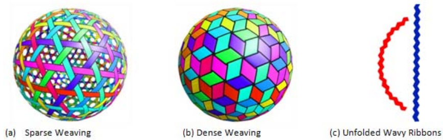
Figure 4 (a) The projection method (PR) can create the same type of "sparse" weaving, by leaving gaps as shown. (b) Using the projection method (PR), we can also create dense triaxial weaving on any regular triangular mesh, as shown. This particular mesh consists of 18 cycles of ribbons. Unfolded versions of these ribbons show that the ribbons are wavy and that there are only two types used in (b). The construction requires 12 from the circular-type ribbon (left) and 6 from the straight-type ribbon (right).
