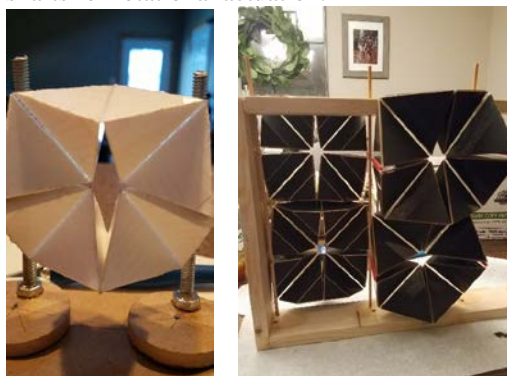
Fig. 3. Rotational actuation of octa-flexagon module and front-to-back array with adjacent modules.
