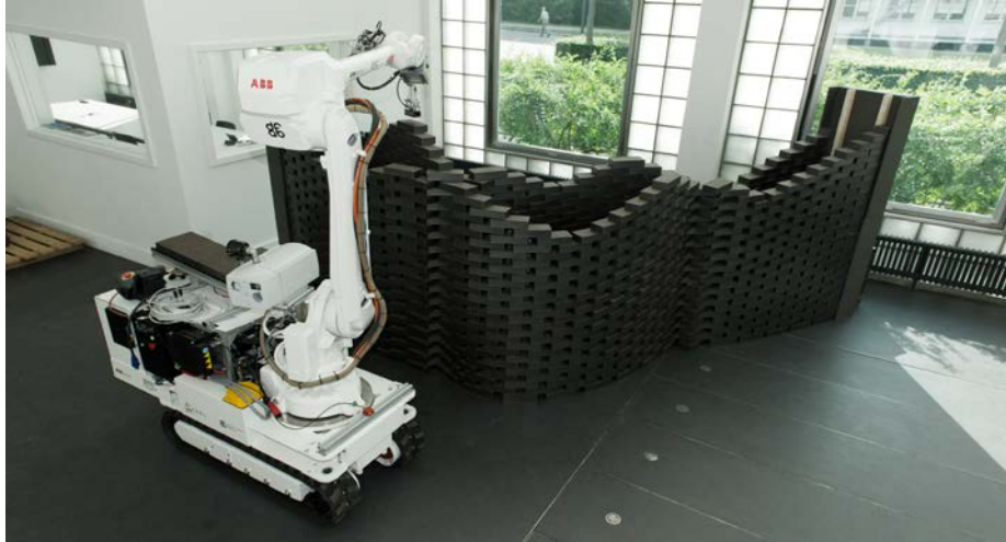
Fig. 10. Experimental result: Double leaf dry stacked brick wall fabricated by the mobile robot. (Photographer: Michael Lyrenmann)
