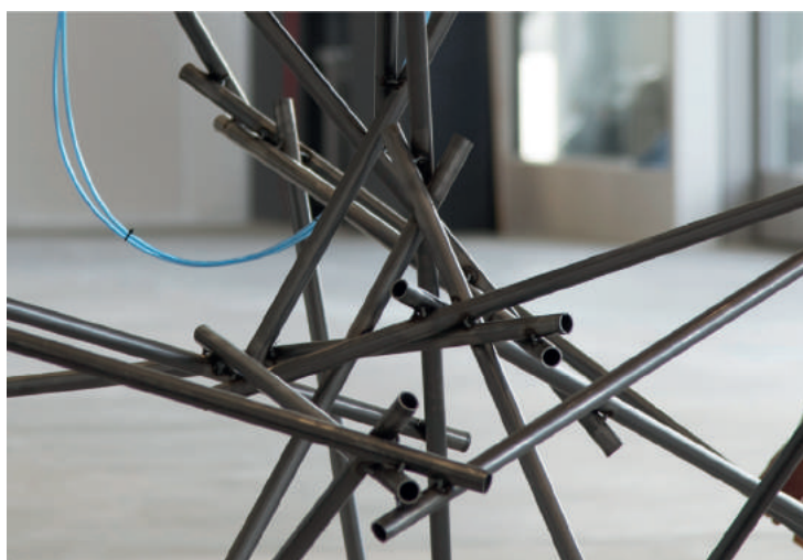
Figure 14: Physical test of a structure in which 14 bars come together in one node.
