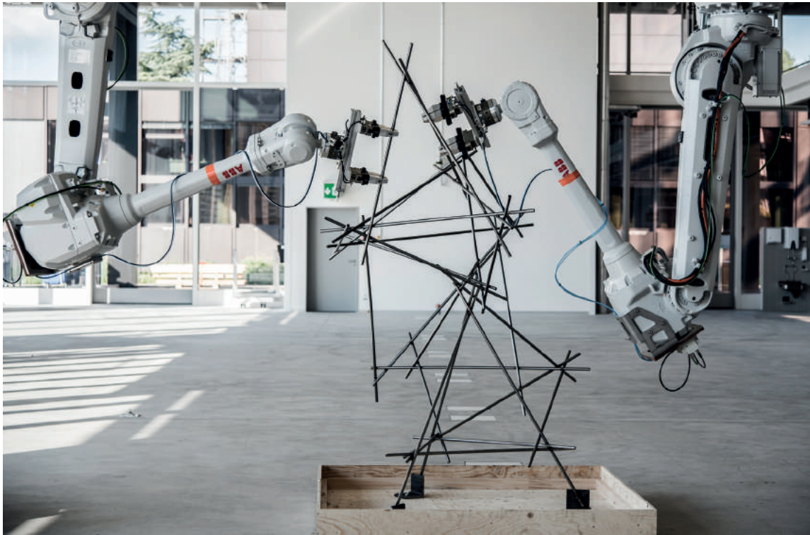
Figure 1: Multi-robotic assembly of spatial structures.
