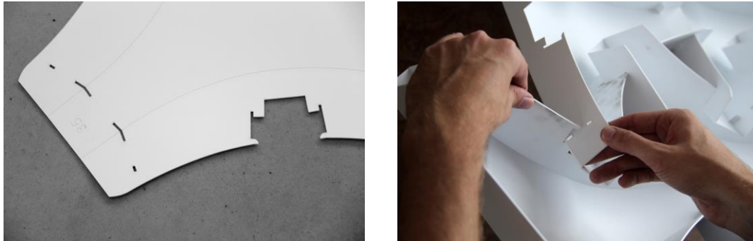
Figure 9: (a) Integrated connections restrain the components in a (b) slide-and-click system.
