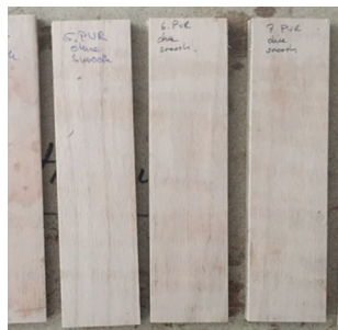
3 Bending test specimens after lamination
