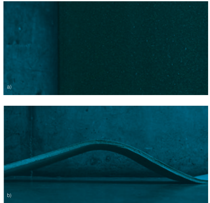
2 Two types of core materials: (a) thermoplastic elastic NFRP core material, and (b) semi-elastic lignocellulosic oriented fiber core
