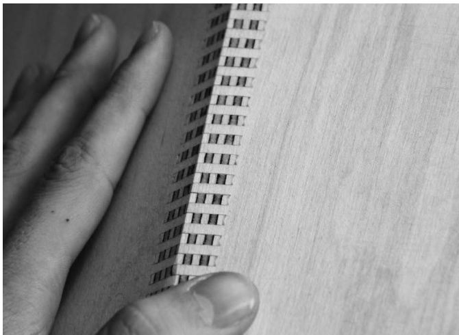
4a Finger Joint Fabrication – Curved finger joints connecting two plates
