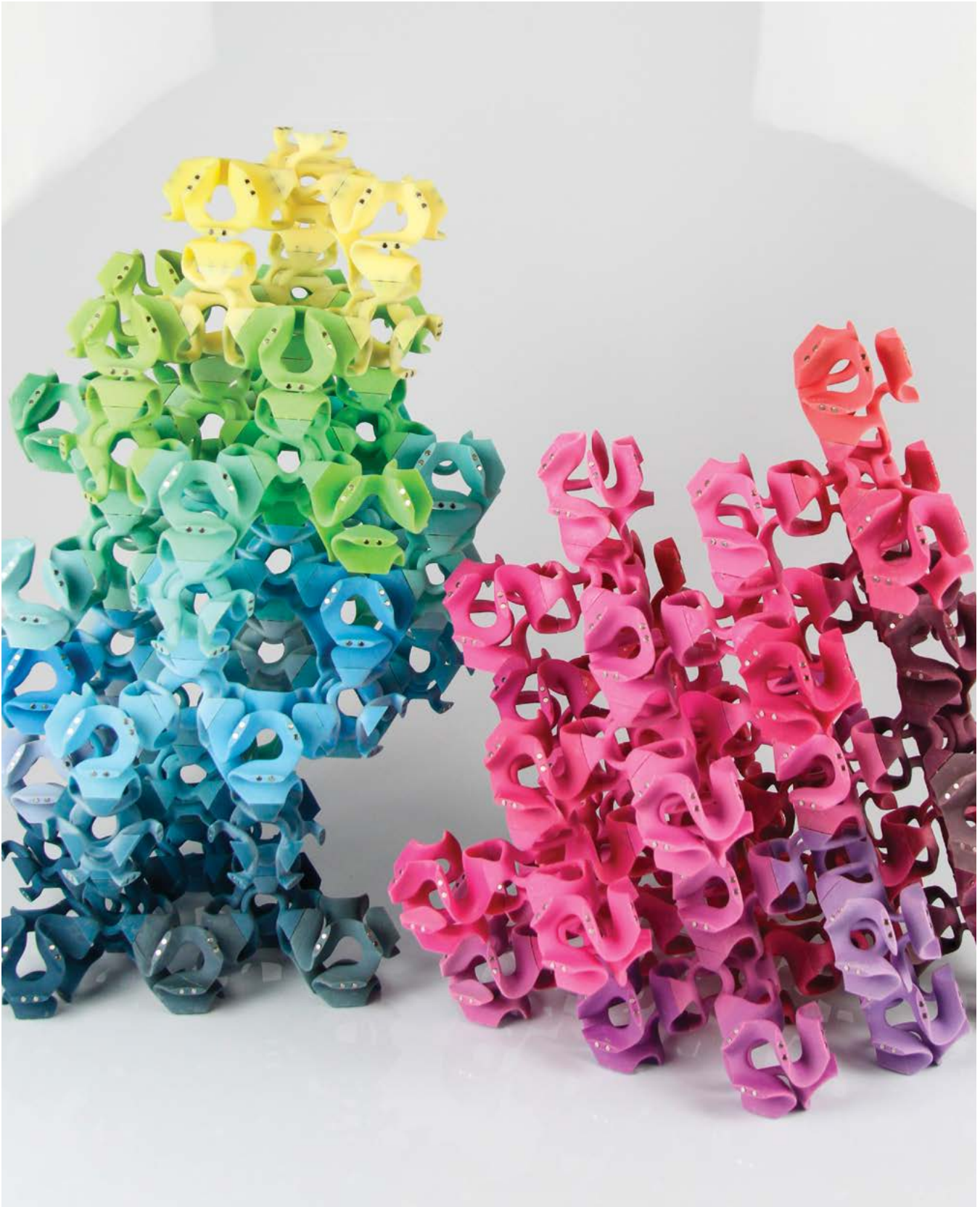
12 3D Printed piece developed out of the gaming platform. The units have been printed separately and magnets have been added to the face connections to allow the growth of the voxel structure.
