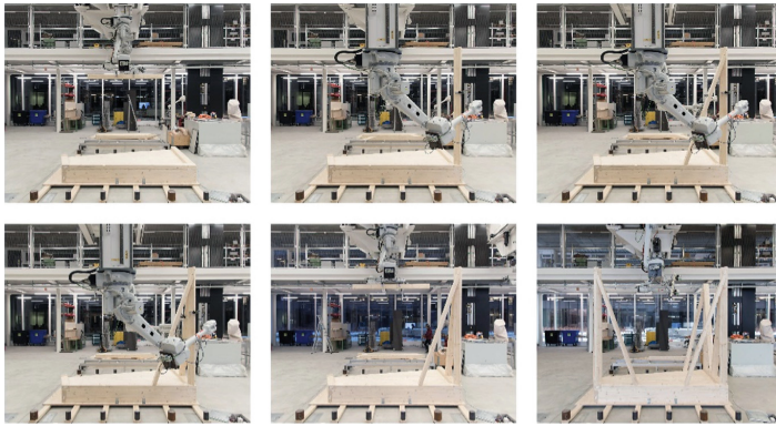
Fig. 3. Cooperative assembly sequence
