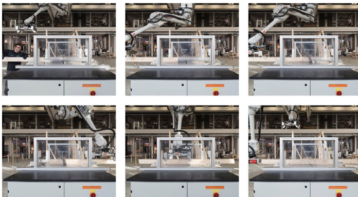
Fig. 4. Beam Cutting and Detailing Sequence: 1. The robot positions the beam and saw executes the first cut. 2. The robot positions the beam and the saw executes the second cut. 3. The beam is repositioned and the robot proceeds to mill and drill the required detailing.
