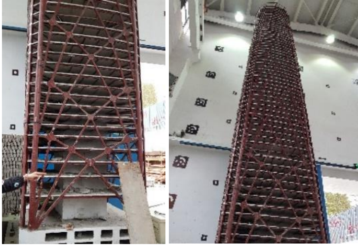
Figure 125: CITIC tower miniature at the shaking tables laboratory of Tongji University
