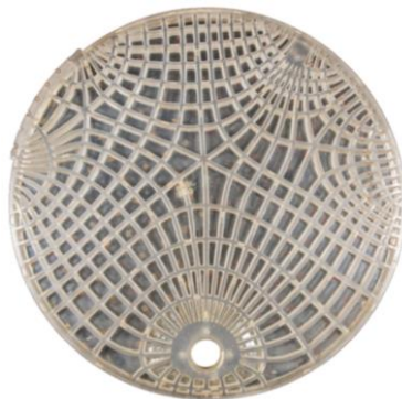
Figure 83: Scale model of the slab with isostatic ribs
