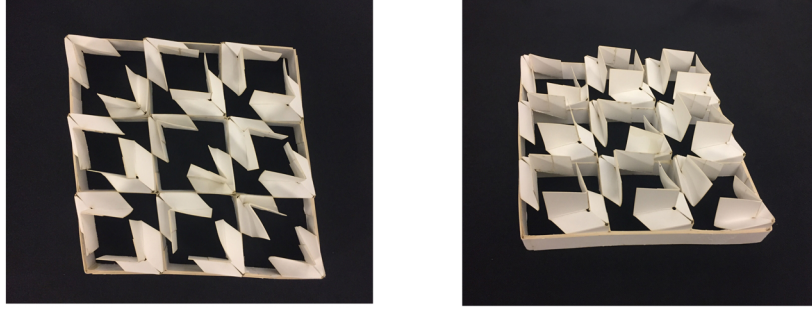
Figure S5: Photographs of the 3 \times 3 PERMuTE material provide a top-down view (left) and a three-quarters perspective view (right). Notice that material has been removed at vertices to avoid the effects of material stretching.
