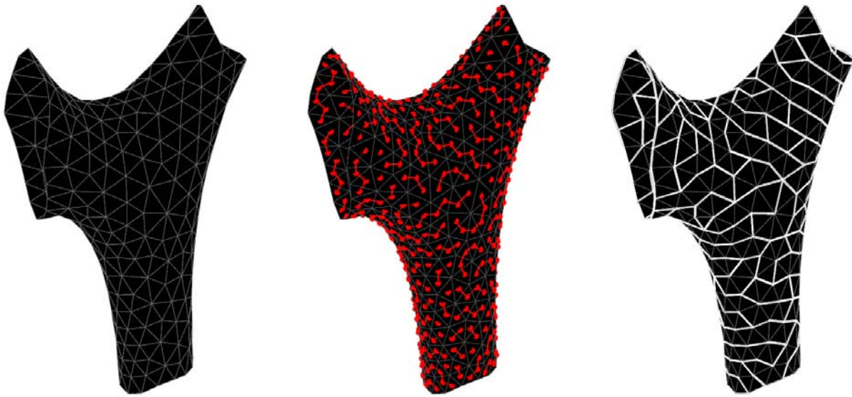
Figure 11: Using a modified Prim's algorithm to produce developable strips of triangles.
