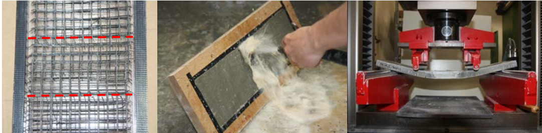
Figure 18, 19, 20: From left to right: Mirco mesh reinforcement in the joint area. This example shows the overlapping version, type B-FU ; the mortar sealing is washed out before casting the joint; four point bending test setup. The sample illustrates the ductile behaviour of the micro mesh reinforced concrete.
