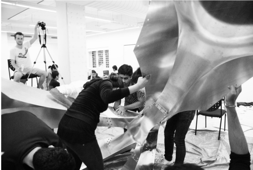
Figure 11: 2m long aluminium CFPs folded and assembled in 6 hours by a group of 15 students
