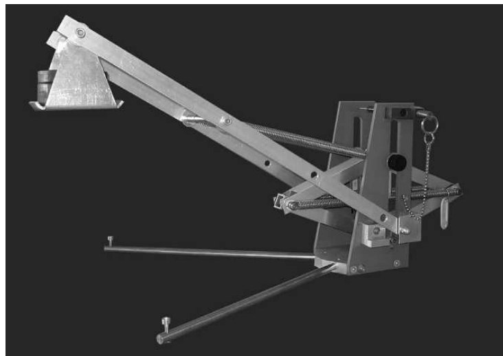
Figure 10 – Practical implementation of a gravity equilibrator using the parallelogram storage spring principle with zero-free-length spring [32].
