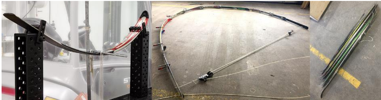
Figure 3. Bending stiffness tests on a ski (left) and on a nominal arch (centre). Folded arch (right).
