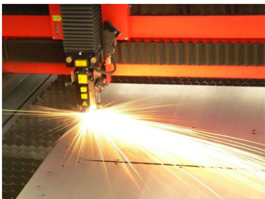
Fig 8:Epilog Laser Cutter and Engraver at work. Image courtesy Fedtech.
