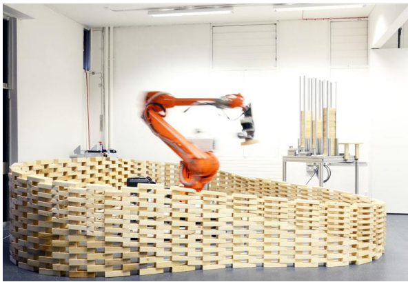
Fig 12: Robotic construction of a parametric brick wall. Image courtesy ETH.
