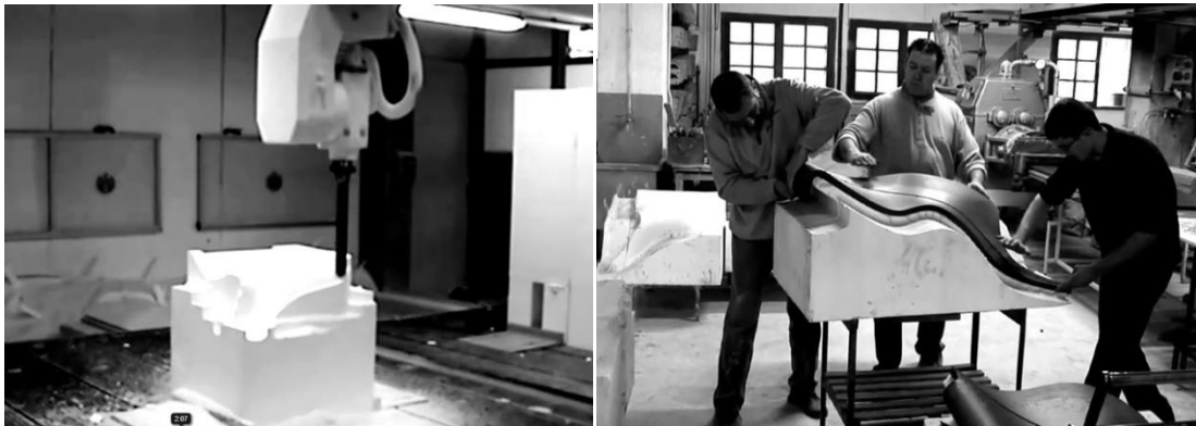
Fig 10: Digital Fabrication of Moulds for Villa Nurbs Facade. Images courtesy Coud9.
