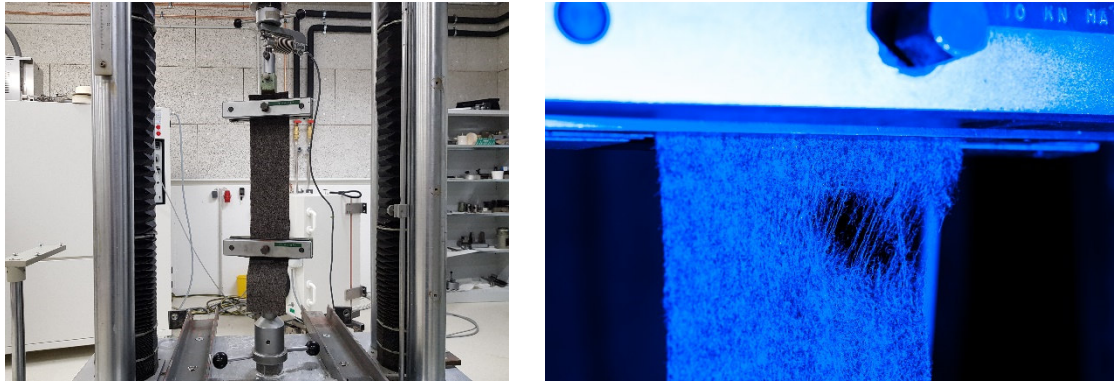
Figure 5: Uniaxial tensile test of membrane strips
