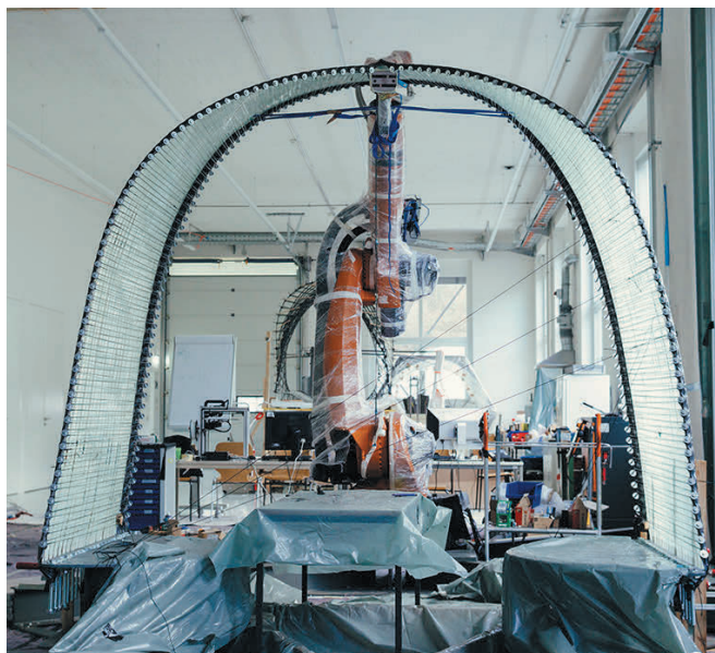
7 An elastically bent glass fiber sheet is incrementally reinforced through a process of winding volumetrically with glass and then carbon fiber.
