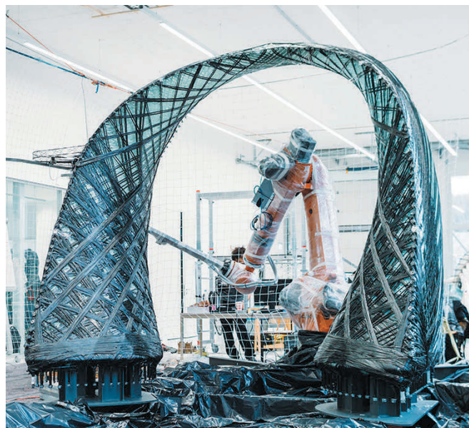
7 An elastically bent glass fiber sheet is incrementally reinforced through a process of winding volumetrically with glass and then carbon fiber.
