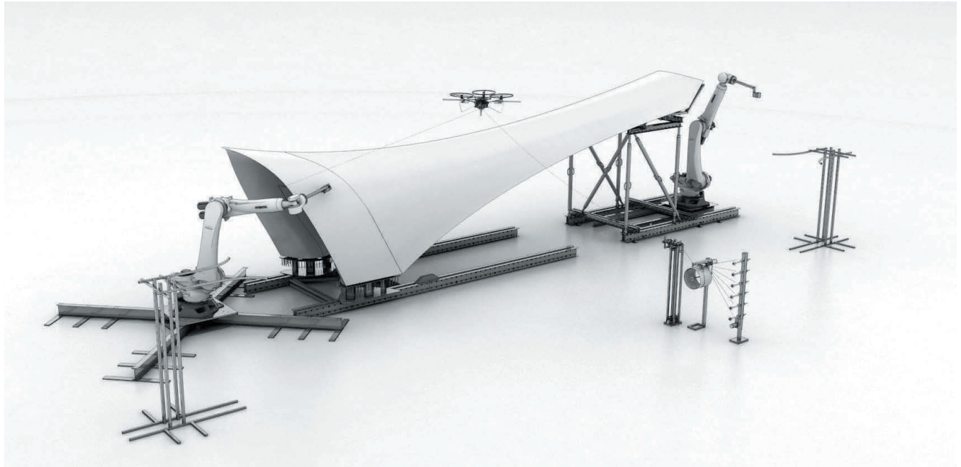
4 Fabrication setup with industrial robots, UAV, landing stations and a tension mechanism
