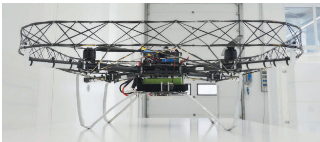
5 Interactive Fiber exchange through passing fiber carrying winding effector between robot and UAV
