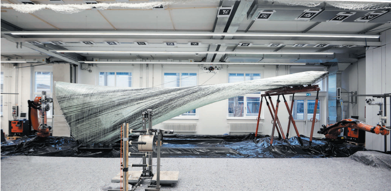
12 Fabrication setup with completed glass fiber form and early carbon fiber placement, the tension mechanism is shown in the foreground
