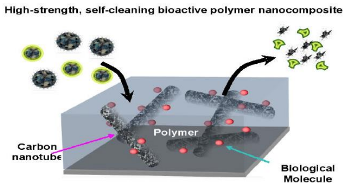
Figure 3-19 Self-Cleaning Enzyme Nanotube- Polymer Composite material.
