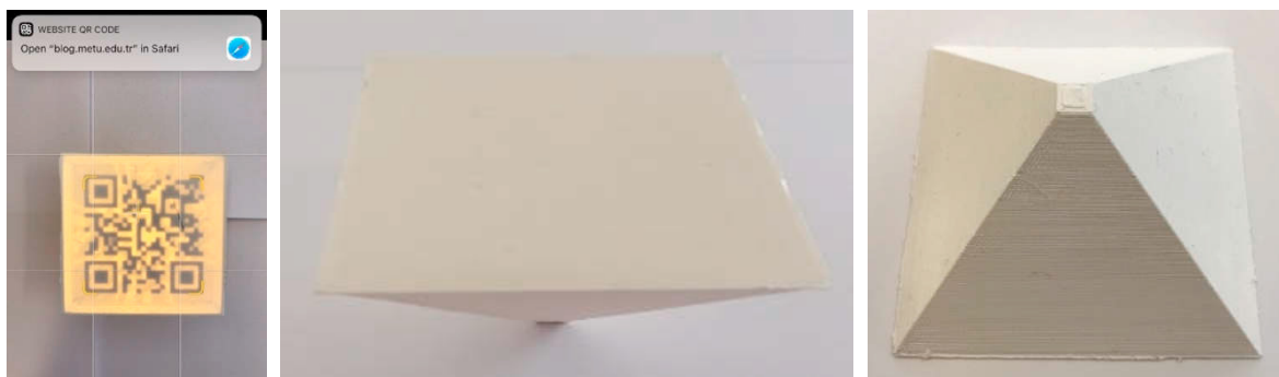
Fig. 5. Scanning of the QR Code embedded into the solid.
