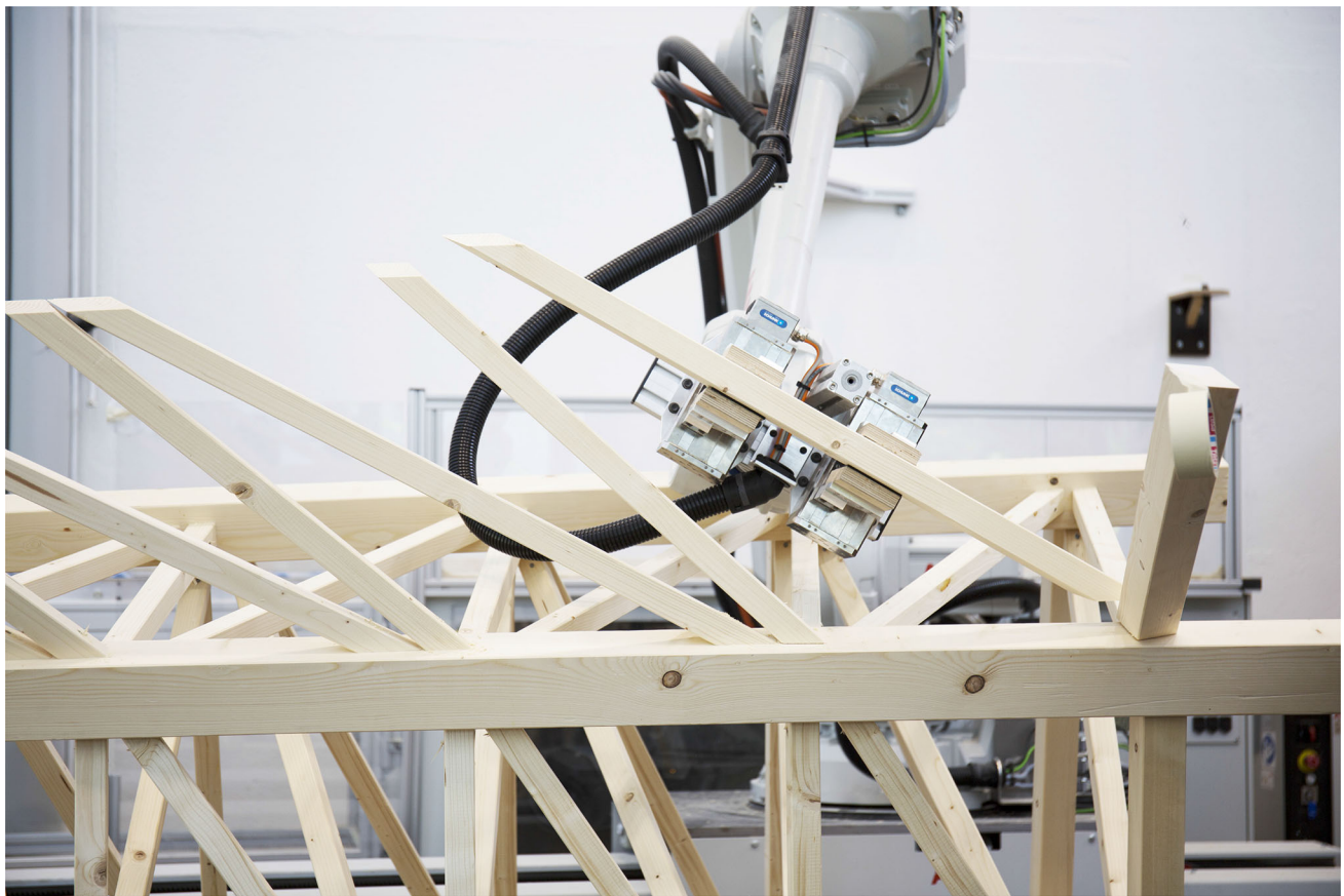
Fig. 9 Assembly sequence of wooden slat in truss element: the beam gets placed in the truss, where it is fixated manually
