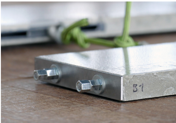
Figure 22: Dry-fit connection method. The magnitude of the prestressing is controlled by the monitoring of the screw nut rotations
