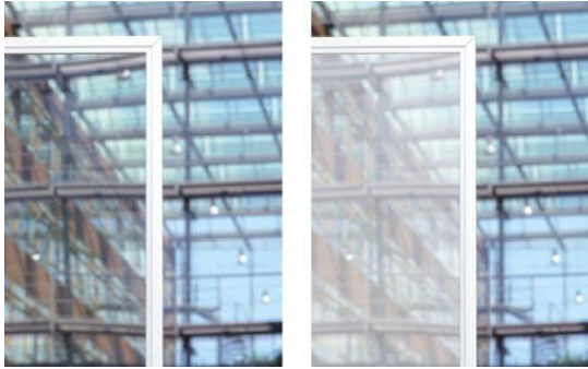
Figure 24. Thermo tropic glazing (off and on state) [52].
