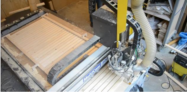
Figure 14: The CNC-router mills five holes in each lath.
