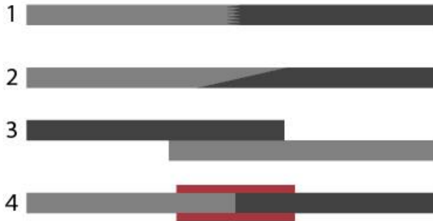
Figure 7: Comparison of extension techniques. (1) Finger jointing, used in Mannheim Multihalle, Weald & Downland and Savill Garden (2) Scarf jointing, used in Weald & Downland and Savill Garden. (3) Bypass jointing, used in segment lath and gridshell.it's pavilions (4) Lap-jointing, used to repair broken laths in Mannheim Multihalle
