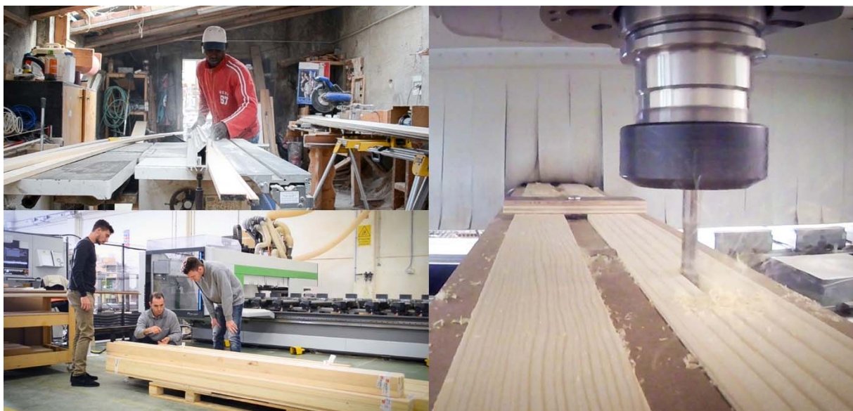
Figure 3: preliminary and industrial processing; right, the milling of two laths in the jig. [Image: A. Liuti]
