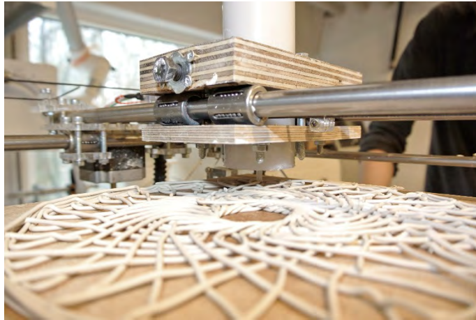
Figure 5. The code informs a RapMan 3d printer to print directly in porcelain layer by layer. The concept of the module and the parametric setup are based on this principle of a continuous curve.
