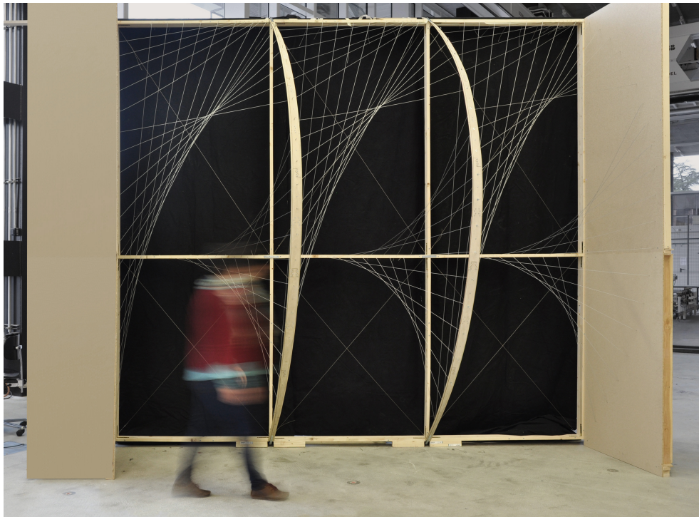
Figure 5.18: 1:2 scale structural prototype of an exemplary portion of the sun-shading structure.
