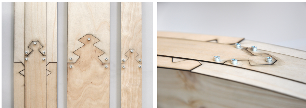
Figure 5.12: Investigation on the geometry of the dove tail joints and their distribution in the beams.
