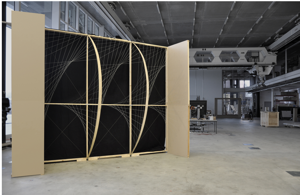
Figure 5.10: 1:2 scale structural prototype of an exemplary portion of the sun-shading structure.
