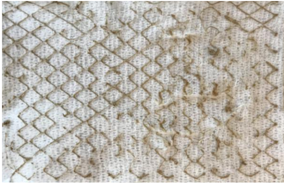
Figure 4- 9 Showing the Result of Trial 1: First Layer Infill Width: 0.42 mm (0.0165 inch), First Layer Infill Height: 0.2 mm (0.008 inch), Extruder Temperature: 215°C (419°F), Heat Bed Temperature: 60°C (140°F)
