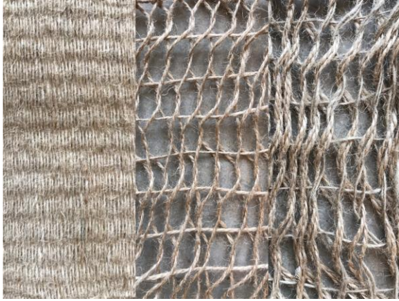
Figure 4- 5 Woven Fabrics Made of Jute Fibers: Plain Weave, Single Gauze Weave and Double Gauze Weave (Horizontal Warp Direction)
