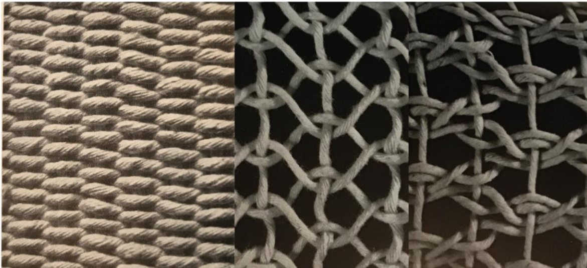
Figure 4- 2 Left: Weft-Faced Plain Weave pg.86 Center: Plain Alternating Gauze Weave. pg.183 Left: A Complex Alternating Gauze Weave pg.185 , Adapted from “The Primary Structures of Fabrics” by Emery, Irène, 1966, Washington: Textile Museum. Copyright 1966 by the Textile Museum
