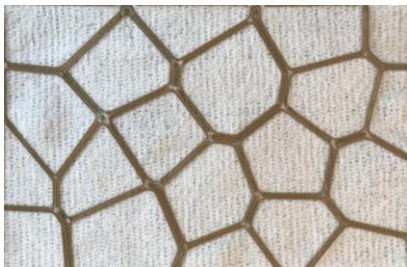
Figure 4- 14 Showing the Result of Voronoi Tool Path
