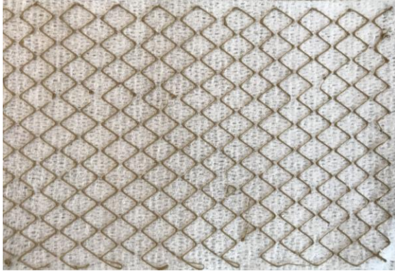
Figure 4- 11 Showing the Result of Trial 3: First Layer Infill Width: 0.8 mm (0.032 inch) ,First Layer Infill Height: 0.4 mm (0.016 inch). Extruder Temperature: 215°C (419°F), Heat Bead Temperature: 60°C (140°F)
