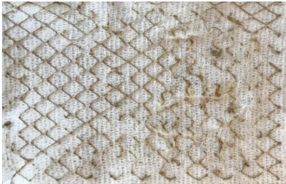
Figure 4- 10 Showing the Result of Trial 2: First Layer Infill Width: 0.42 mm (0.0165 inch), First Layer Infill Height: 0.2 mm (0.008 inch), Extruder Temperature: 230°C (446°F), Heat Bed Temperature: 85°C (185°F)
