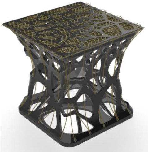
Figure 6- 6 Connection of Fabric to Frame
