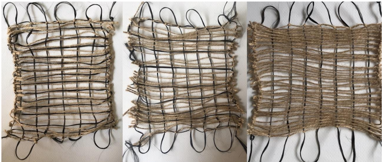
Figure 4- 6 Left: Warps: 9 x CFRP Wefts: 16 x CFRP, 32 x Jute, Center: Warps: 9 x CFRP Wefts: 10 x CFRP, 38 x Jute, Right: Warps: 9 x CFRP, Wefts: 0 x CFRP, 48 x Jute (Vertical Warp Direction)
