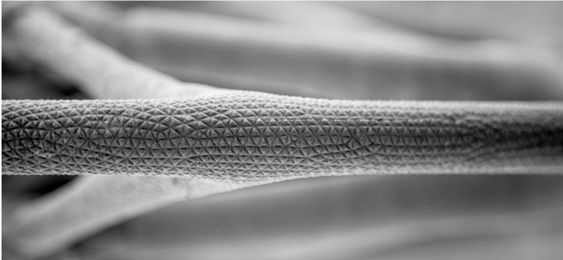
Figure 5.21: High resolution texture on the surface of the skelETHon . This texture maximises the contact area with the waterproofing concrete skin. (dbt, PCBM, ETH Zürich, 2017)
