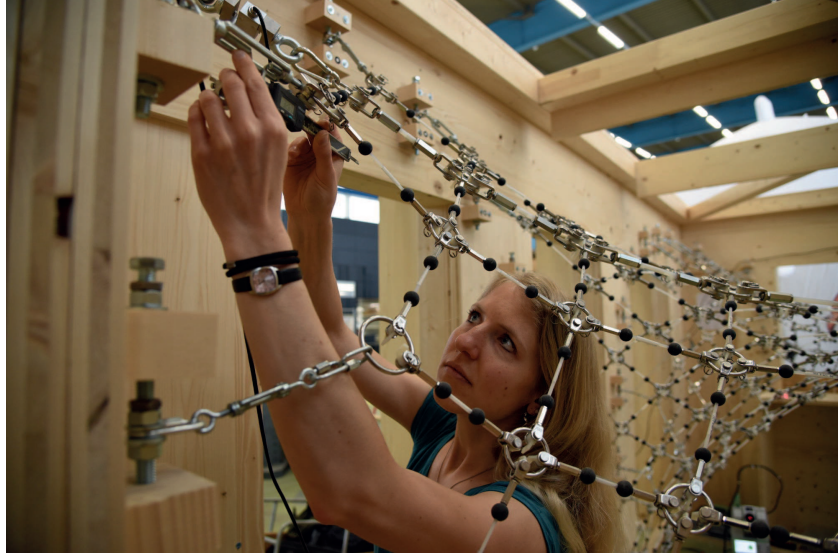
Figure 13.4: Manual application of control actions: Measuring the changes in lengths of the boundary edges by calipers and adjusting the turnbuckles to apply the computed control inputs.
