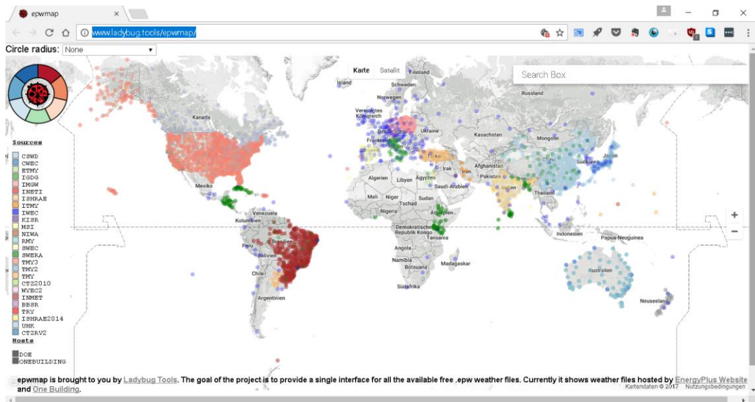
Figure 4-2: Ladybug can import weather files from the internet with a single click (source: http://www.ladybug.tools/epwmap/ ).
