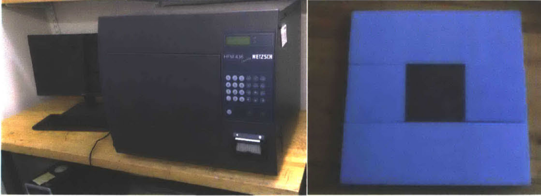
Figure 4.12: Heat Flow Meter (HFM) 436 Lambda by Netzsch (Left) and initial test specimen of 10cm by 10cm by 2.5 cm aluminum block surrounded by styrofoam blocks for the entire specimen sized as 30 cm by 30 cm by 2.5 cm.
