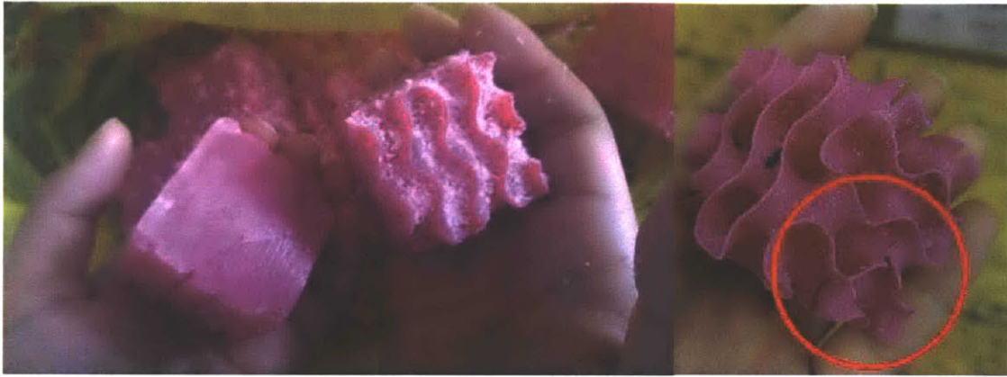
Figure 3.8: Issues with post-printing process required for the 3D printed models by Stratasys's 3D printer: Wax to be removed (Left) and cracks made for prints with thinner gyroid surface during cleaning process (Right)
