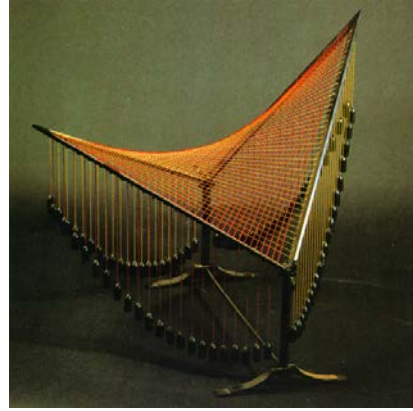
Fig. 2.2: String surface model of a hyperbolic paraboloid [23]
