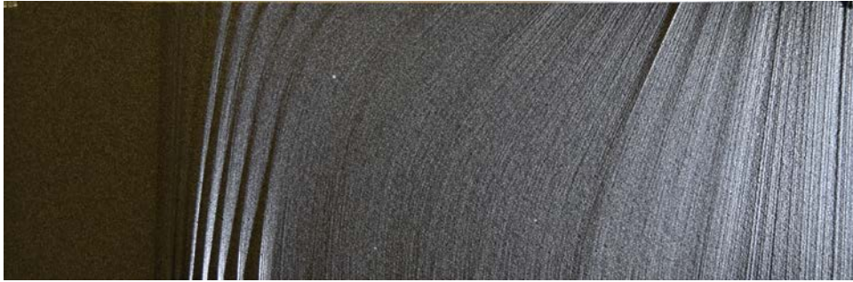
Fig. 3.28: Cutting example with inadequate relation between left and right path-positions in the beginning: high force on left (top in picture) side controls the speed, while the wire at the right (bottom in picture) side melts the foam, since it is moving too slow. Additionally oscillation errors occur (see Section 3.4.1)
