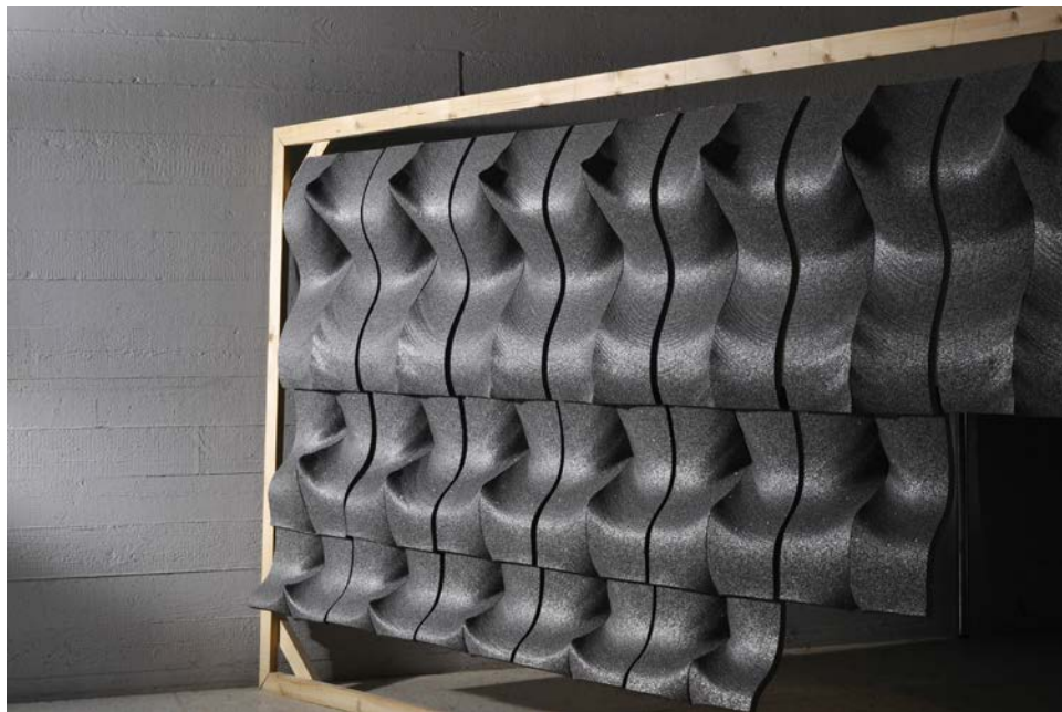
Fig. 4.9: Final prototype of Group 3: The panels with varying element size overlapped vertically.
