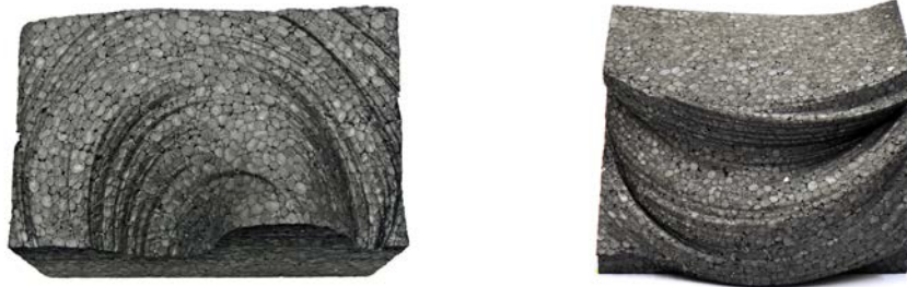
Fig. 3.29: Cutting tests, in which the tension was not at a constant level, leading the material to melt. The resulting surface pattern clearly exhibits the wire's traces, however is hardly controllable
