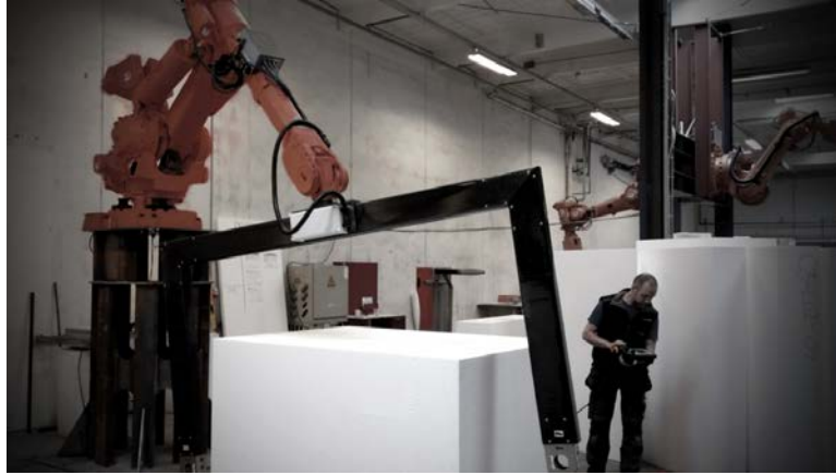
Fig. 2.14: Robotic arm cutting large scale moulds at Odico Formworks Robotics [54]
