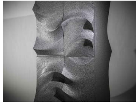
Fig. 4.20: Photo of manual tests, flipping cutting direction
