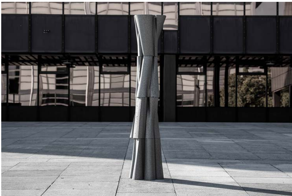
Fig. A.5: Final column of Group 4: The elements were cut along the transverse direction of the column through a single cut
