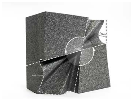
Fig. 4.2: Variation possibilities on one element: angle, depth and path-curves
