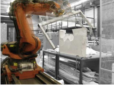
Fig. 2.9: Set-up used for fabricating Persicope by Matter Design Studio [42]
