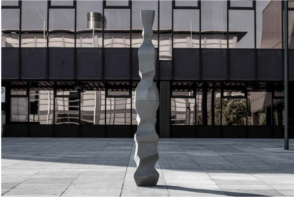
Fig. A.4: Final column of Group 3: The elements were produced by cutting twice on each of the four sides of the column, creating surface intersections
