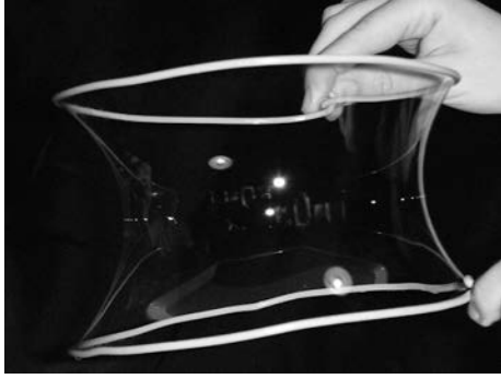
Fig. 2.17: Minimal surface of revolution [74]
