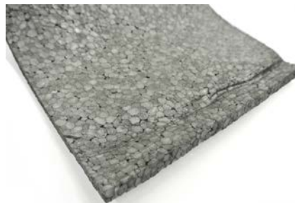
Fig. 3.30: Cutting example in which through joint acceleration limits the tension force could not successfully be targeted resulting into melted material
