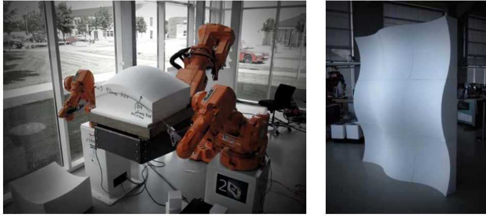
Fig. 2.15: Project Bladerunner : Tri-robot hot-blade cutting configuration (left) and fabricated prototype (right) [56]
