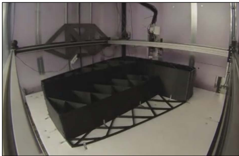
Figure A.8 - Kamermaker by DUS Architects ( 3dprintcanalhouse.com , 2014)
