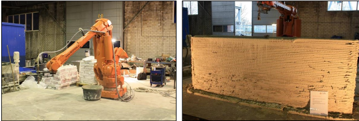
Fig A.25 – Robot arm (left) and 3D printed wall (right) by CyBe Additive Industries (Anderson, 2015)
