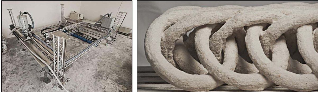
Figure 1.4 - D-Shape by Enrico Dini ( dinitech.it , 2014)
