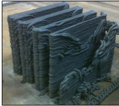
Figure 4.5 – Printed layers collapsed by their own weight (Le, et al., 2011)
