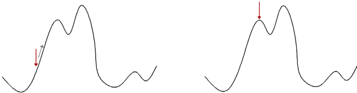
Figure 3.1 – Example of a hill climbing algorithm ending at a local optimum
