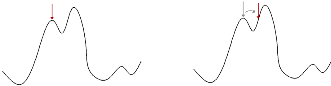
Figure 3.2 – Example of a simulated annealing algorithm jumping out of a local optimum
