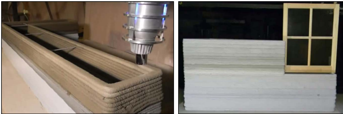
Fig A.23 – 3D Concrete printing by TotalKustom (totalkustom.com, 2014)
