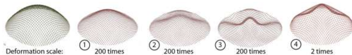
Figure 5.3 6 Left to Right: Intermediary deformation points starting from the undeformed shape up to collapse
