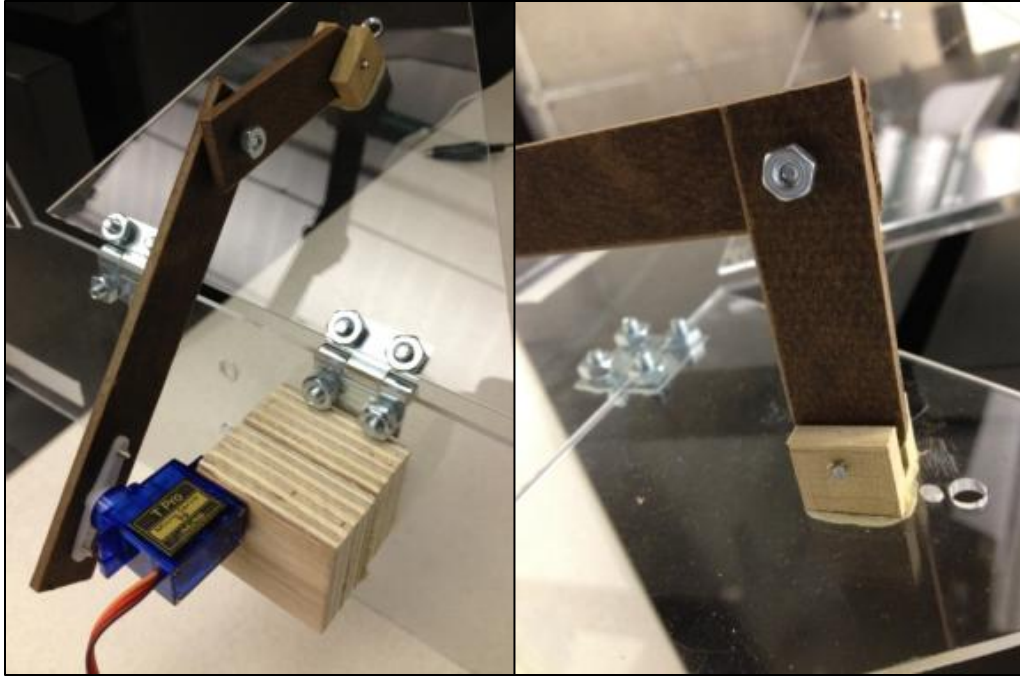
Figure 40 - Views of the automated arm in closed and open states of the module flap. The image shows the joints.
