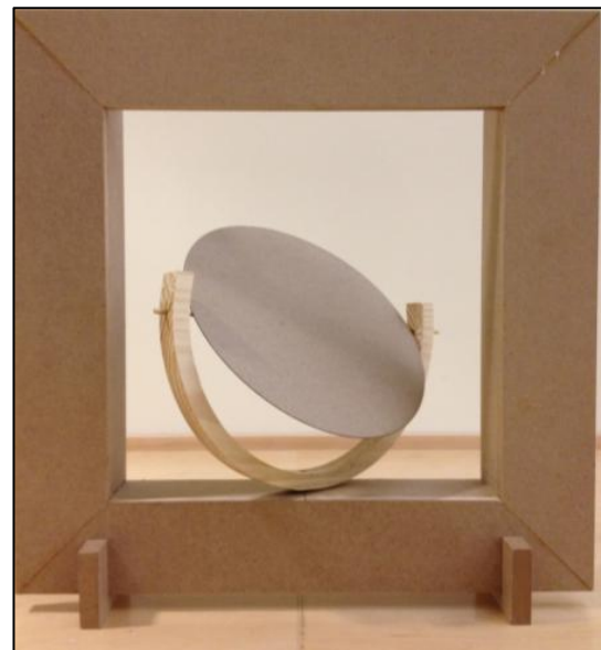
Figure 58- Picture of the circular panel with two axis rotation (Positioned for morning sun). Source: the
