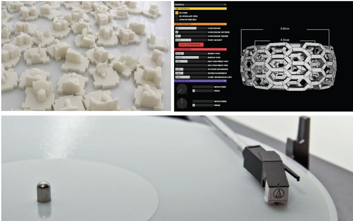
Figure 3-1: Clockwise from upper-left: Fabricate Yourself by Karl D.D. Willis, 3D printed puzzle pieces featuring conference attendees (created with the openFrameworks toolkit, Kinect, and a 3D printer), Cell Cycle Bracelet and Ring creation application by Nervous Systems (created with Cinder toolkit), 3D-printed functional record by Amanda Ghassaei, (created using Processing.)
