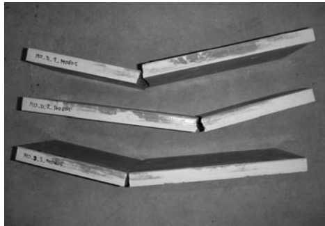
(d) Crack pattern series MO , D: Abrupt failure with no previous crack formation
