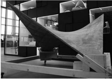
Figure 4.15 Prototype of hybrid cable net and fabric formwork. Photo: Block Research Group, ETH Zurich
