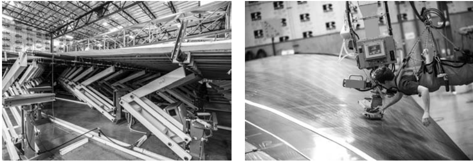
(a) Definition of double curved shape of sails with actuators (b) Lamination process of the sail hydrofoil
