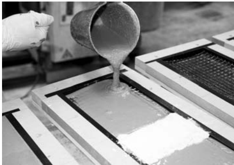
(c) First casting stage—casting of the segments
