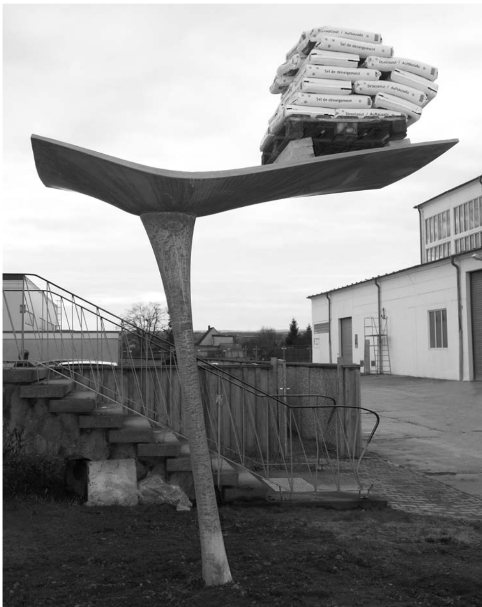
Figure 5.7 Test loading of installed Parapluie prototype as verification of feasibility
