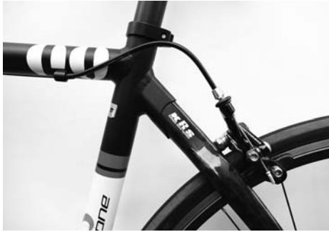
(a) Bowden cables (here on a bicycle) are able to guide magnitudes and directions of force vectors. Although hulls are under compression they never underlie buckling failure
