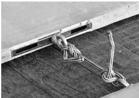
(c) Sliding device with ropes as suspension
