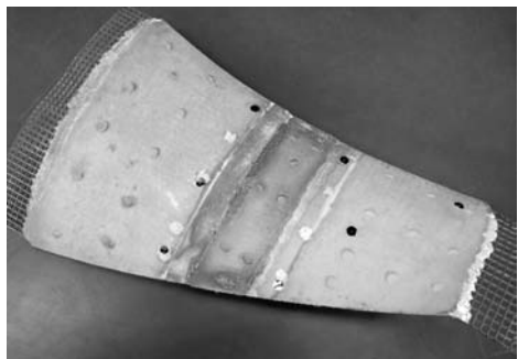
(f) Finished prototype, upper side. The dots on the surface are resulting from spacers
