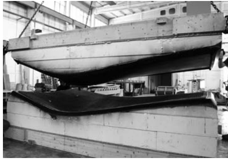
(b) Airtight closing of upper and lower formwork
