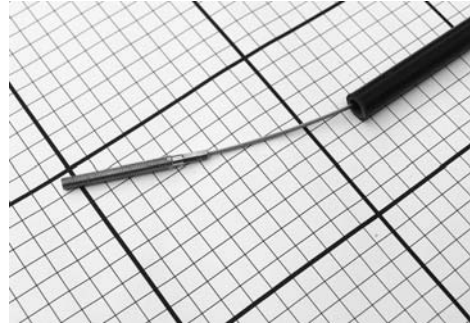
(b) Confected steel wire inside hull for concrete-casting. Both, flexible cable and hull allow curved layout in concrete section
