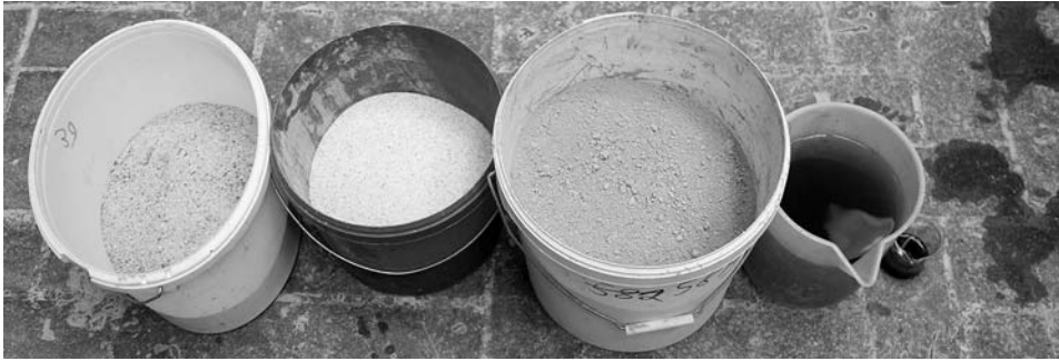
(a) Ingredients fltr: Aggregates 0–2,0mm, 0–1,2mm, cement DUCON 1 , water, plasticiser
