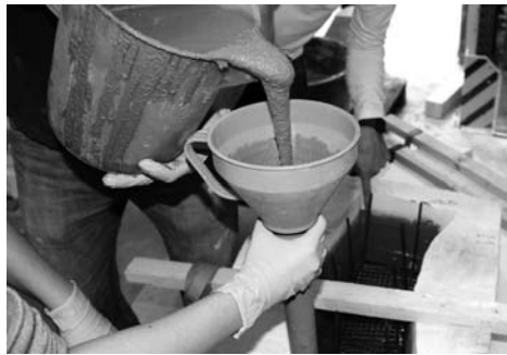
(c) Flowable concrete that 'rains from the trowel' is required for casting process
