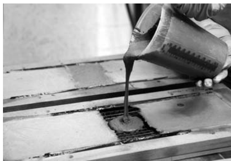
(f) Second casting stage—casting of the joints
