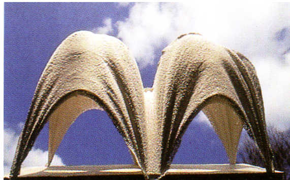
Figure 2.5 Form-Finding Experiments Conducted by Frei Otto and Bodo Rasch at the Institute for Lightweight Structures
