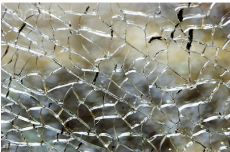
Fig. 5.10 Thermally Cracked Pattern
