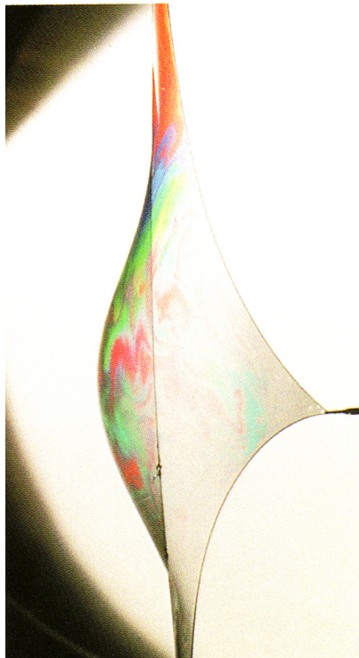
Figure 2.5 Form-Finding Experiments Conducted by Frei Otto and Bodo Rasch at the Institute for Lightweight Structures
