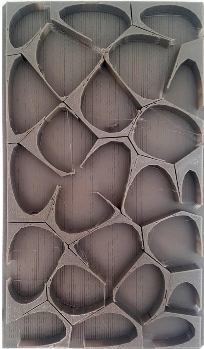
Figure 4-29 This is a top view image of the 3D printed copy of the voronoi prototype model. This model was printed from the University of Guelph's Digital Design Lab. This is an example of the versatility of parametric technology in terms of its capabilities of producing quick 3D prints directly from the Rhinoceros 3D and Grasshopper software's (Source: Author).
