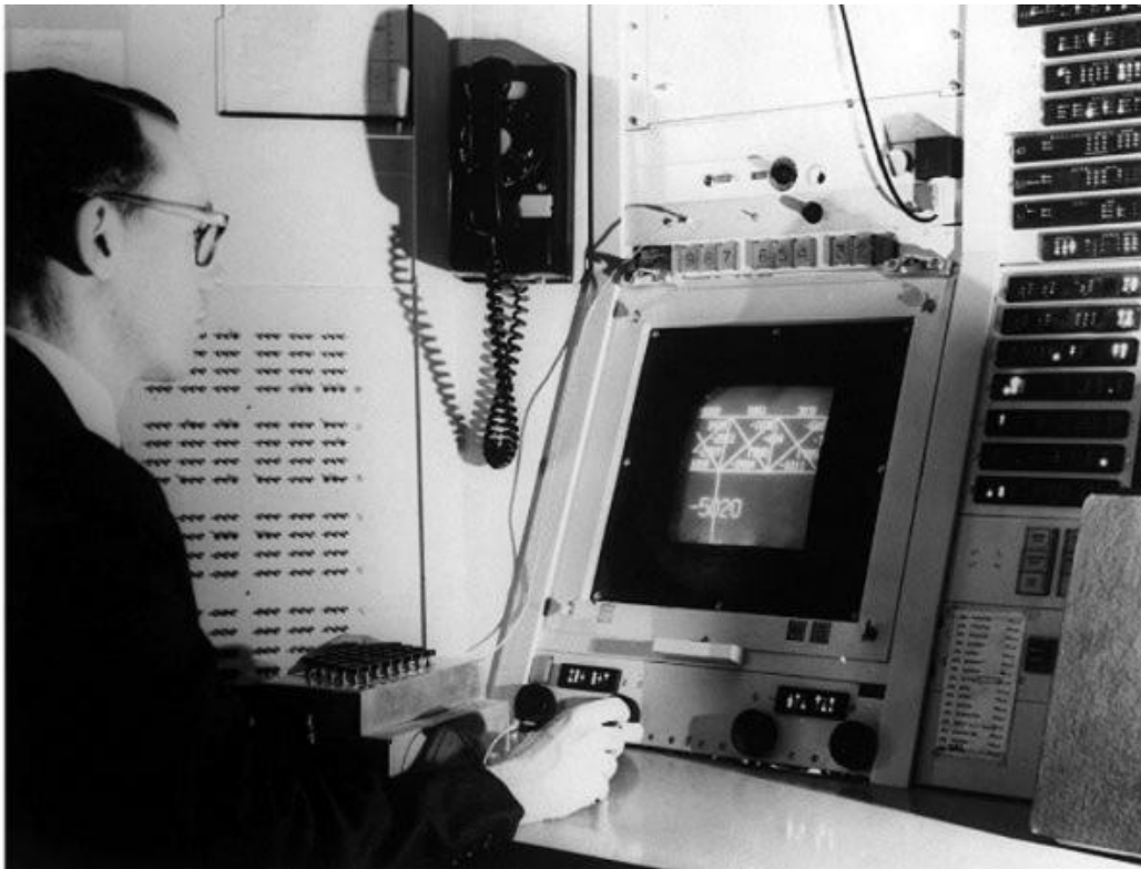
Figure 2-3 This is an image of a designer using the TX-2 Operating System demonstrating the Sketchpad in use. The designer is using the light pen to create drawings projected onto the screen. To control the functions of the drawing, toggle switches are used, see knobs below screen (Sutherland, 1980).
