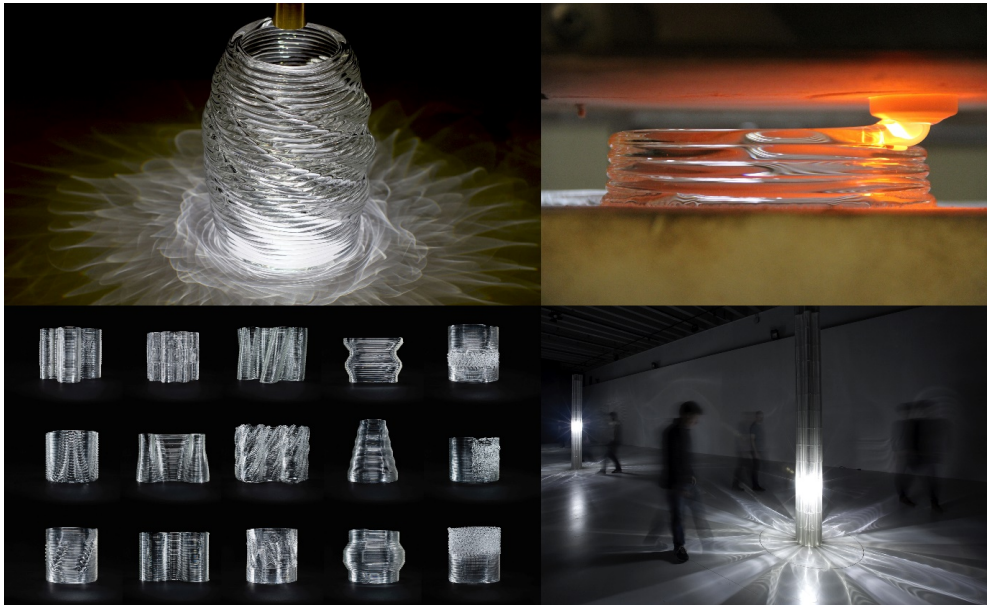
Figure 3: Additive manufacturing of optically transparent glass by the Mediated Matter Group, MIT Media Lab. Glass object with caustic pattern (top left), 3D printing process (top right), variety of printable objects (bottom left) and glass column with inserted light (bottom right) (all images courtesy of the Mediated Matter Group).
