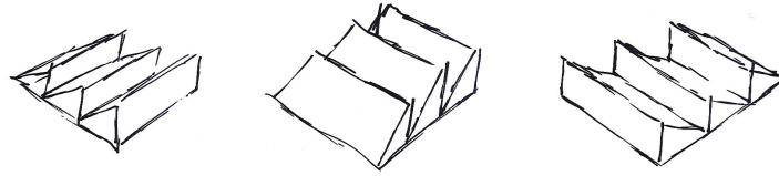
Figure 3.19: Orientations of a sawtooth atrium roof studied.
