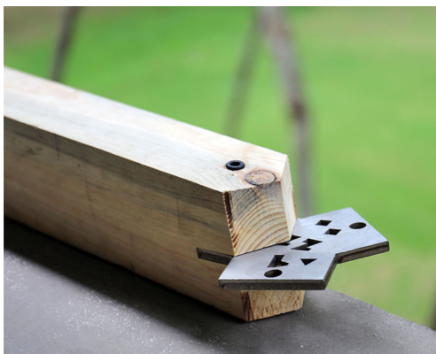
Fig. 10 Joint geometry. The metal plate is not orthogonal to the bar's cross section
